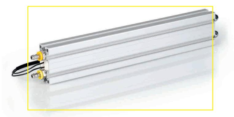
By using water-cooled resistors, the heat development that usually occurs at the location of use is prevented. During braking processes, the electrical drive energy is converted to heat energy. This heat energy is absorbed by the water and can be re-used. Whereas in smaller resistor systems the cooling water is routed directly through the resistor profile, heat exchangers are used in resistors with a power > 50 kW.
