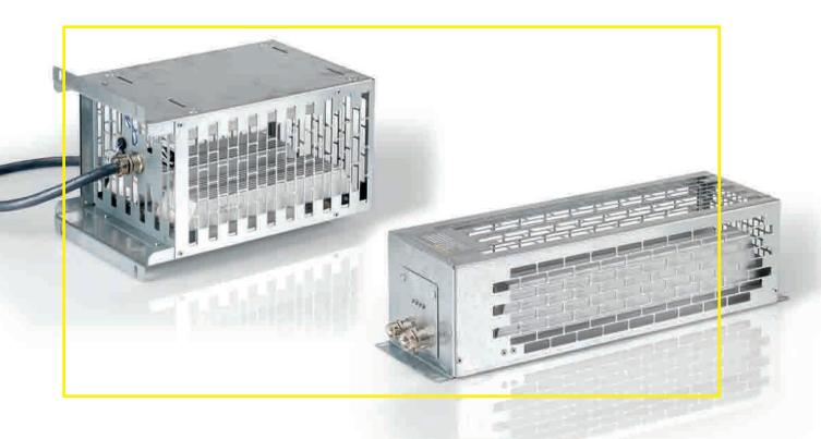
The enclosed resistors can be combined in various housings. Due to their design, the DEG types are also suitable for operation in high humidi condition. In the standard design, the resistors are mounted on a terminal block so that the resulting type of enclosure is IP20 or, with connection box or connection line, IP54. Cable entry is ensured through cable glands.
