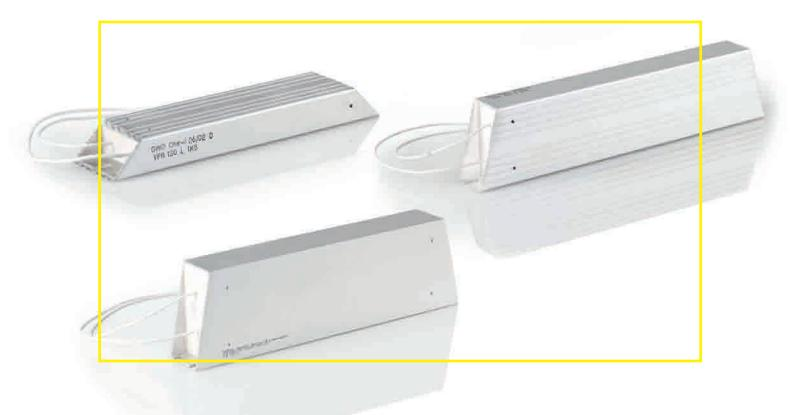
VPR resistors are enclosed in an aluminium profile with PTFE insulated connecting wires of pure nickel. The designs S = vertical and L = horizontal are available.
